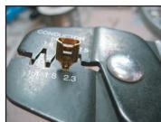
Crimp upper tabs of terminal over stripped part of wire using 2.3 setting on crimper.
