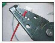
Strip approx. 1cm of wire insulation off both ends of the wire using 20 setting on stripper.
