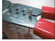
Crimp upper tabs of terminal over stripped part of wire using 2.8 setting on crimper.
