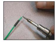
Put 2x heat shrink onto each wire. Tin both ends of the wires as shown.
