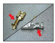
Tin the insides of the battery tab connectors and connector terminals where indicated.
