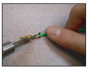
Solder by pressing the wire and terminal together with soldering iron. One of each terminal type per wire.
