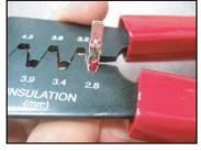
Crimp lower tabs of terminal over insulation part of wire using 2.8 setting on crimper.
