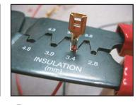
Crimp lower tabs of terminal over insulation part of wire using 3.4 setting on crimper.
