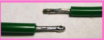
3. Tin the exposed wire with solder (infuse the wire with solder)
