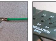
Solder by pressing the wire and terminal together with soldering iron. One terminal per wire. Add solder if neccesary.
