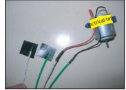
Tape connector leads to motor leads and test with control system. Swap leads if neccessary.
