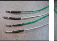
Using a heat gun, "shrink" heat shrink is soldered onto terminal.
