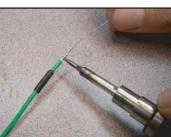
Tin both ends of the wires as shown.
