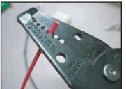
Strip approx. 1cm of wire insulation off both ends of the wire using 20 setting on stripper.
