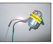
Solder connector lead with corresponding motor lead. Heat shrink over solder joint.
