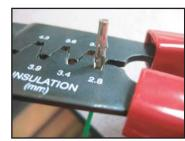
Crimp upper tabs of terminal over stripped part of wire using 2.8 setting on crimper.
