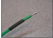
A tined piece of wire looks like this. Put 1 piece of heat shrink onto each wire.
