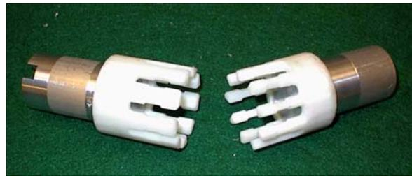
(d) Perpendicular adjustment 3-D printed coupling with adapters for the test setup
