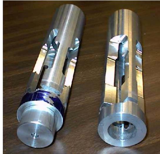
(b) Aluminum coupling machined from bar-stock
