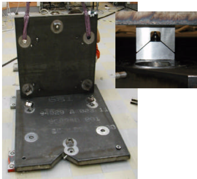
Figure 16: (a) Prototype canoe ball kinematic coupling interface plates for industrial robot base mounting. Production design would machine grooves directly to robot foot, and place balls in floor-mounted baseplate. (b) Close view of single coupling with tooling ball for calibration.
